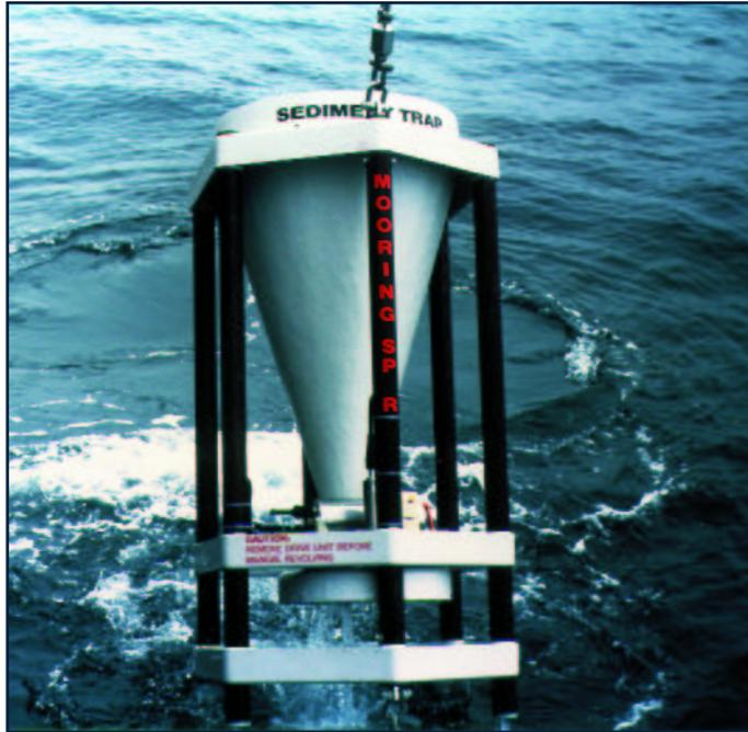
Sediment traps are used to investigate the vertical flux of particles in a water column for deployment in both oceans and inland waters.
