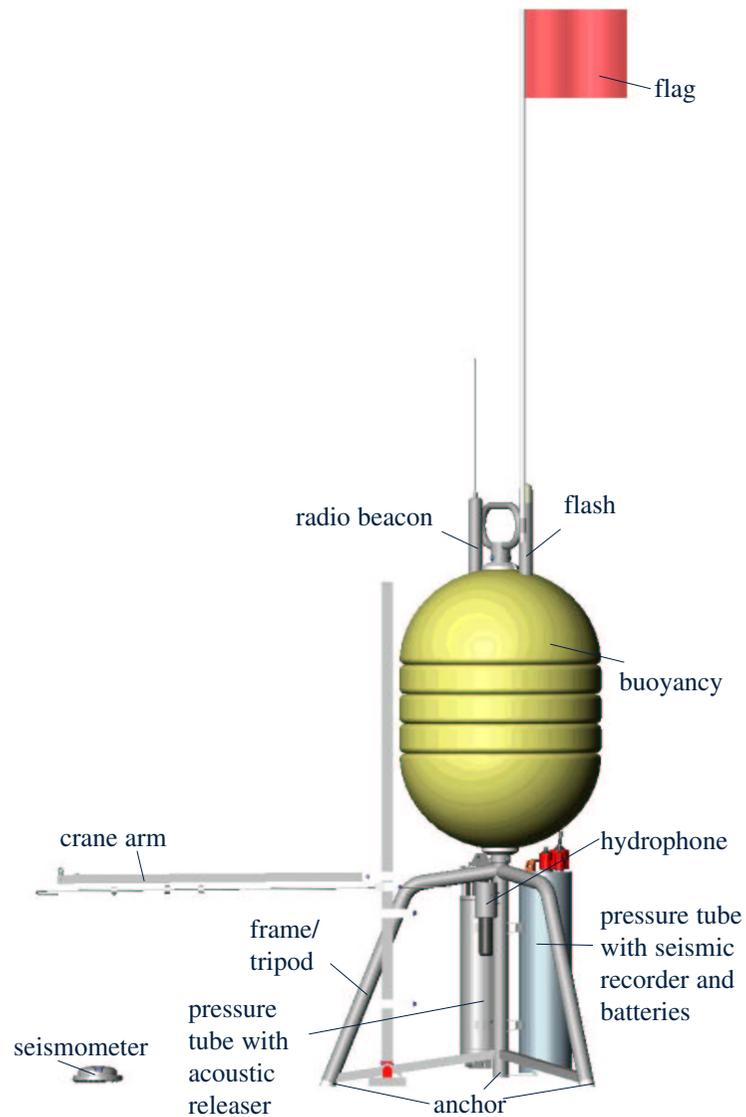
The OBS is heaved overboard from a research vessel, sinks down to the sea floor grace to its anchor weight and stays there autonomously.
