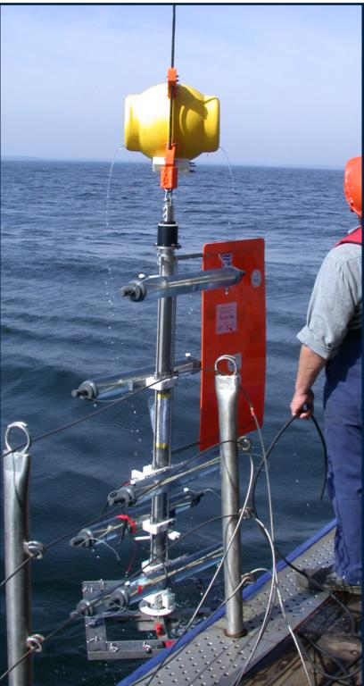
The six transparent water bottles vertically adjustable are aligned with the current by a current vane.
