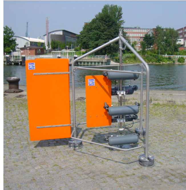
Dr. M. Zabel (University of Bremen): BWS for biogeochemical investigation of the water-sediment surface
